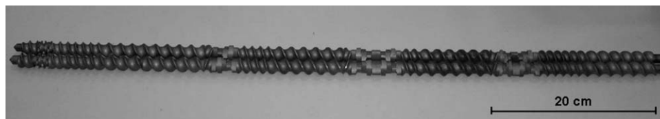
Figure 2. The screw configuration used for melt compounding.
